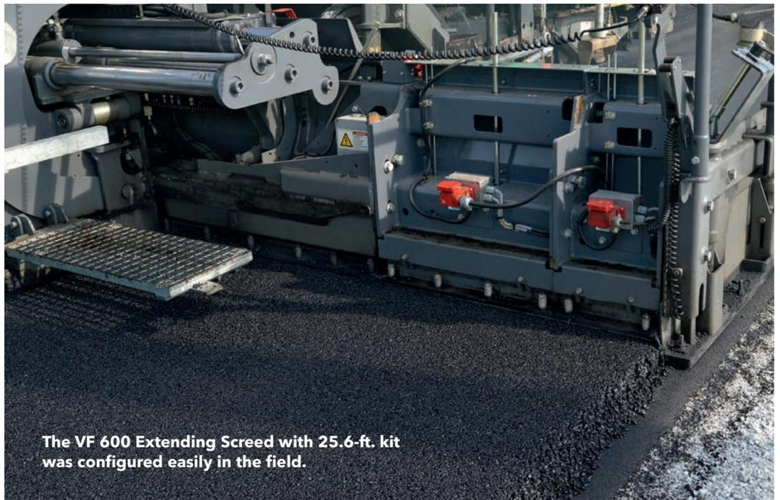
**The VF 600 Extending Screed with 25.6-ft. kit was configured easily in the field.**
